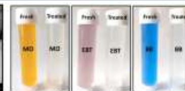
Images of fresh samples and treated sample for adsorption of dyes using MIL-53 (Al)
